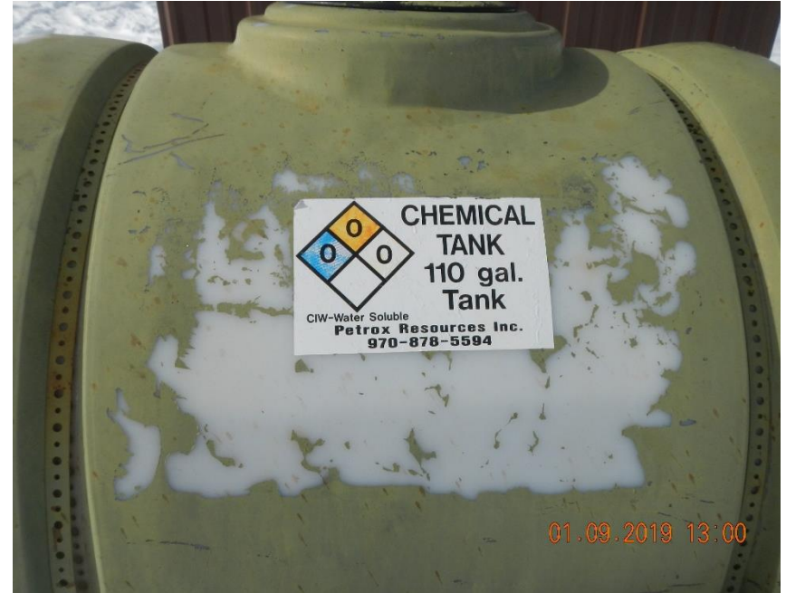
NFPA placard for corrosion inhibitor chemical container has zeros for all fields.
