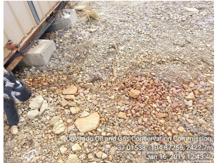
Photo 2 stained soil in front of 1" drain to sep
