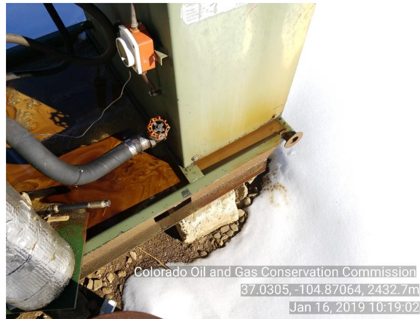
Photo 4 Fluid spilling onto snow off motor skid
