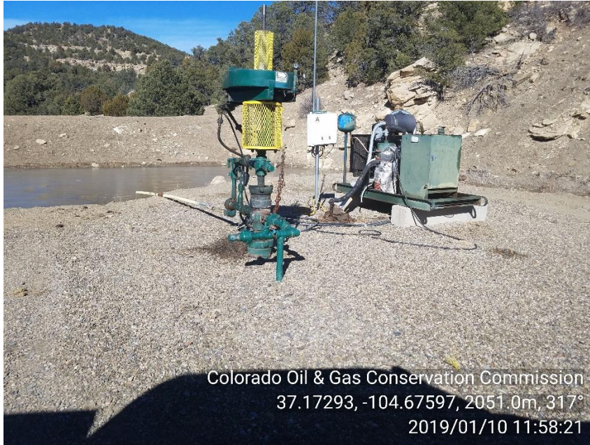
PHOTO 3: STAINED SOIL UNDER DRIVEHEAD MOTOR AND AROUND ENGINE SKID
