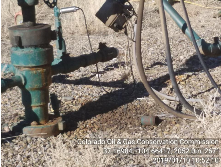
PHOTO 3: STAINED SOIL UNDER DRIVEHEAD HYDRAULIC CONNECTIONS AT WELLHEAD
