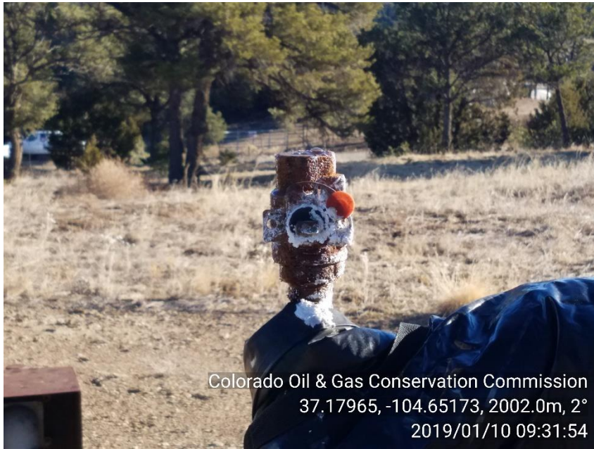
PHOTO 5: APPEARS TO BE LEAKING VALVE ON SALES LINE ATTACHED TO WELLHEAD
