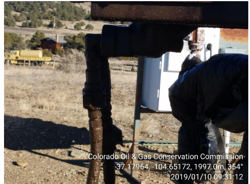
PHOTO 4: HYDRAULIC LINES ARE SATURATED INDICATING A POSSIBLE LEAK
