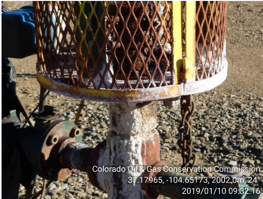
PHOTO 7: APPEARS THAT PACKING ON DRIVEHEAD IS LEAKING
