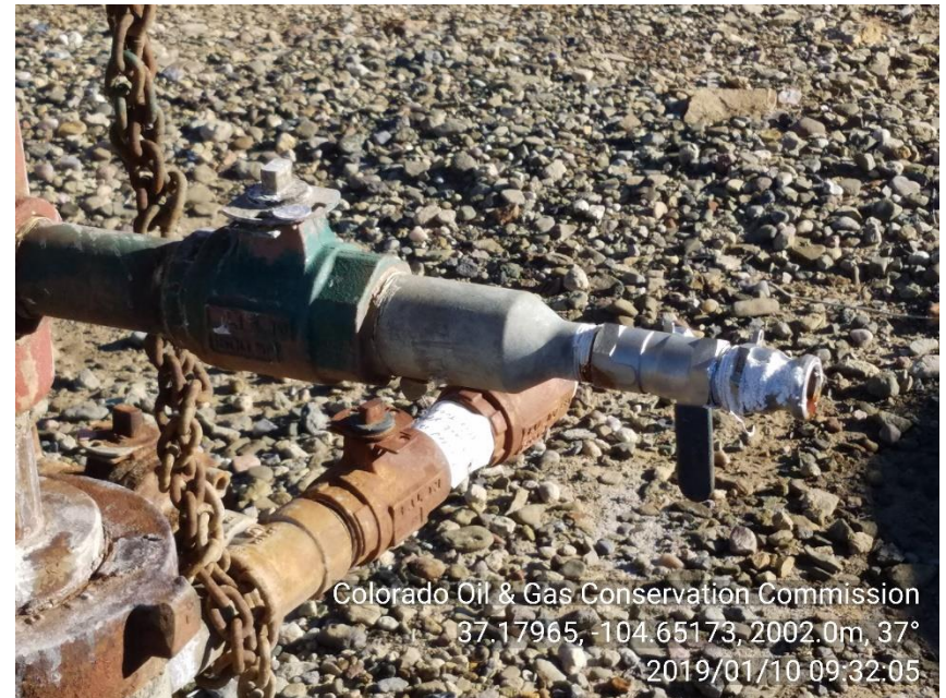
PHOTO 6: LEAKING 1" VALVE ON TBG HEAD
