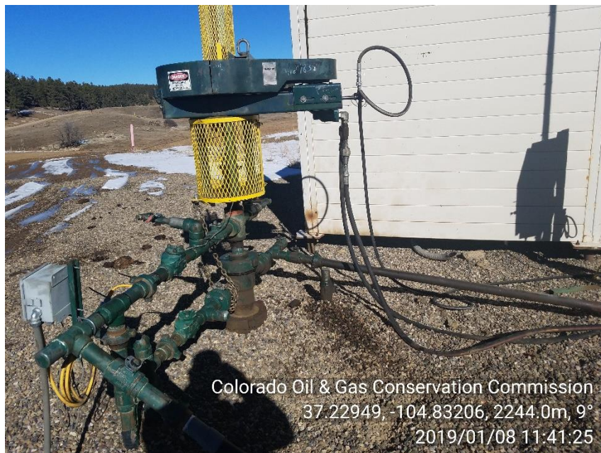
PHOTO 5: STAINED SOIL BENEATH DRIVEHEAD HYDRAULIC LINES
