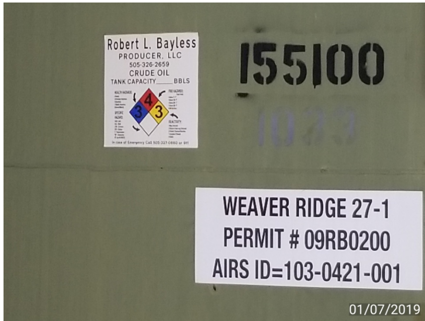
Photo 5. Missing tank volume capacity of 300 on label.
