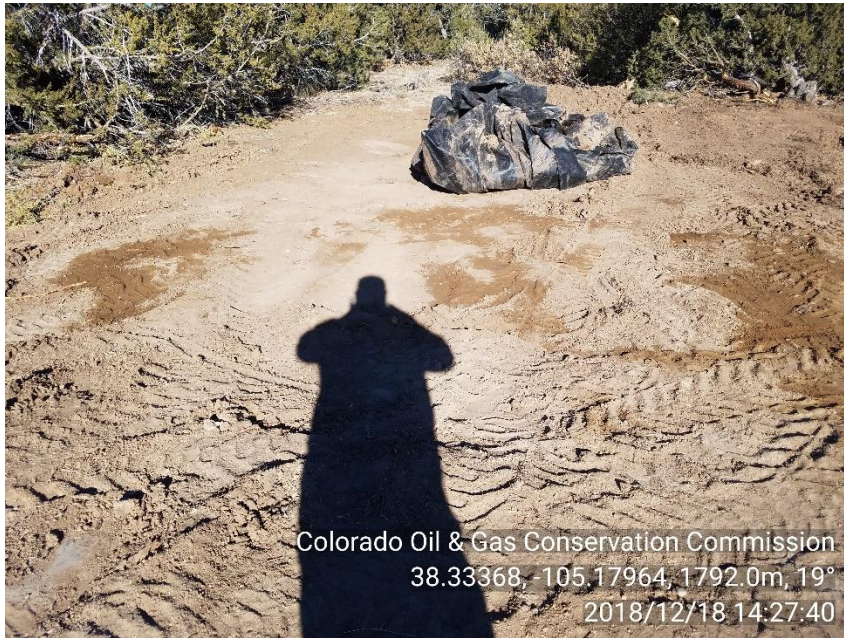
PHOTO 9: STAINED SOIL WHERE FUEL TANK WAS DURING DRILLING OPERATIONS
