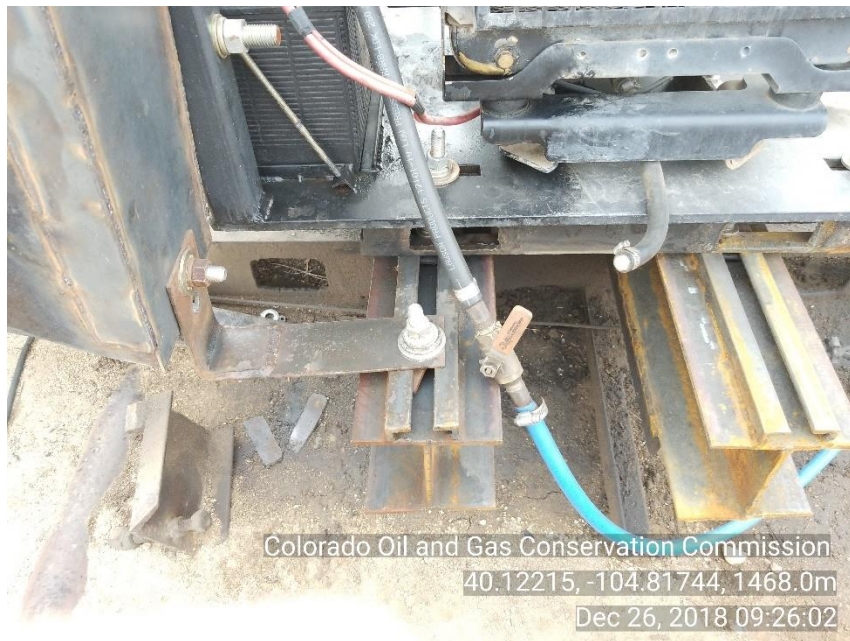
Photo 5 fuel gas leak on VLV
