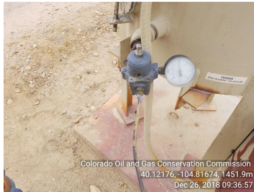
Photo 8 Leaking fuel gas line to ECD
