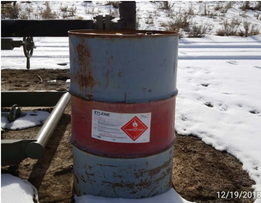
Photo 3. Barrel stored on location without secondary containment.
