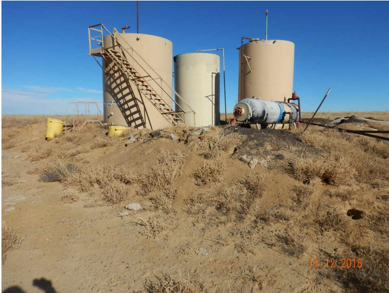
Photo 18: Photo taken from the southwest end of the tanks on location, facing northeast. Previous inspection documented incomplete signage on tanks, including NFPA diamond labeling, and required operator to implement proper signage. Photo shows additional signage has not been implemented.
