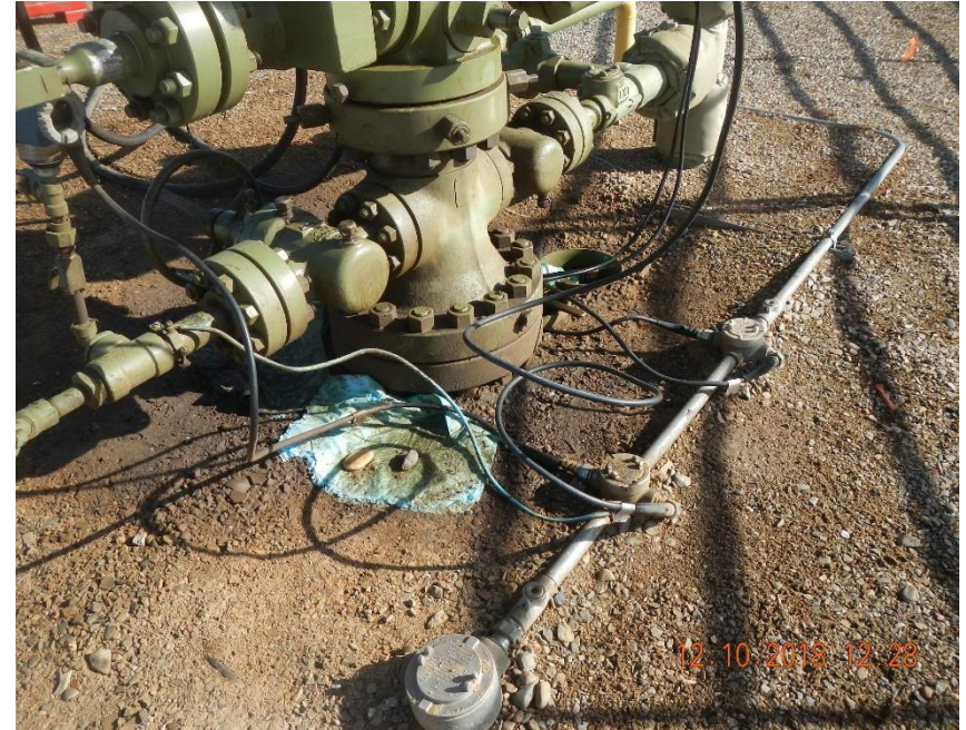
Absorbent wipes and stained gravel near base of well head.
