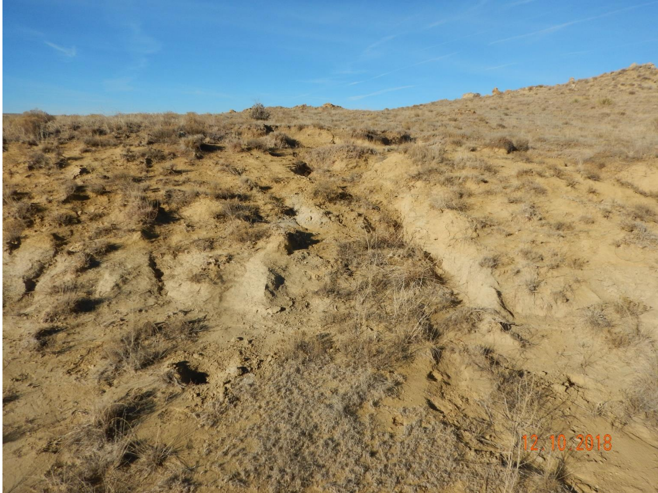
Photo 5: Photo taken from the west end of the pad, facing west. Photo shows vegetation has failed to achieve a uniform establishment, and stormwater runoff has caused erosion degradation on the pad.
