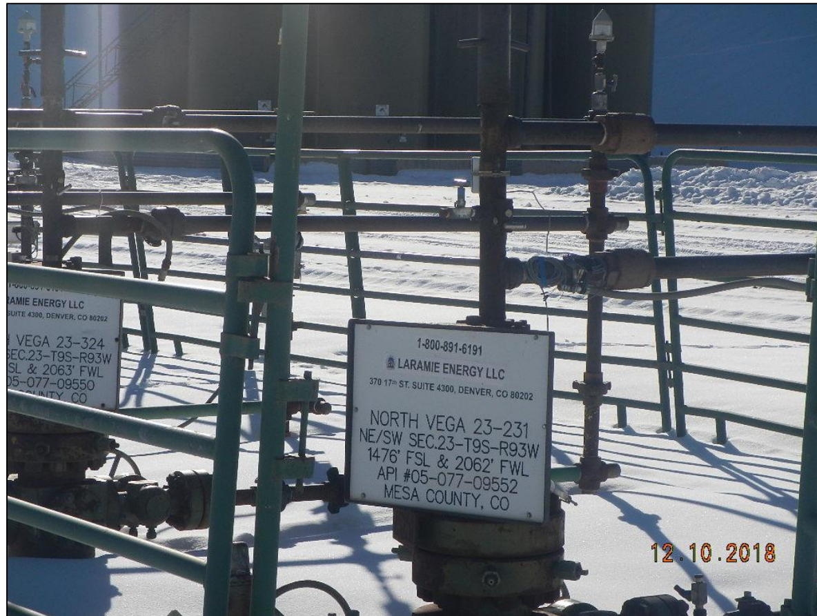
Tank battery sign at well head missing nearest access road information
