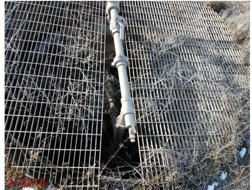
Location Photo #2, Debris in cellar of wellhead.
