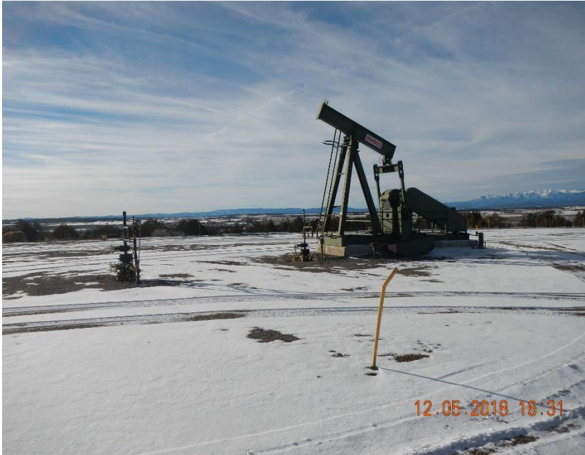
#4-3 and #4-4 well heads. Pump jack on #4-3 was dismantled at the time of this inspection.
