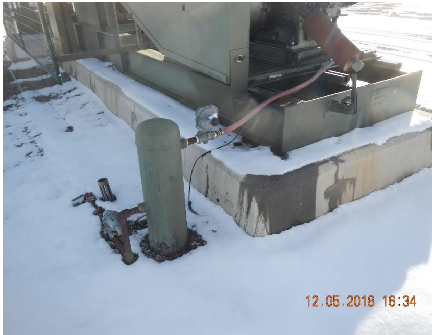
Lube oil leak underneath prime mover on #4-3.
