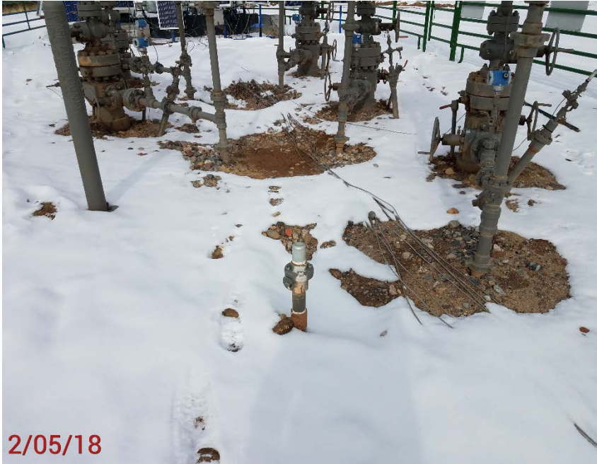
Location Photo #3, unmarked flow line riser near wellheads.
