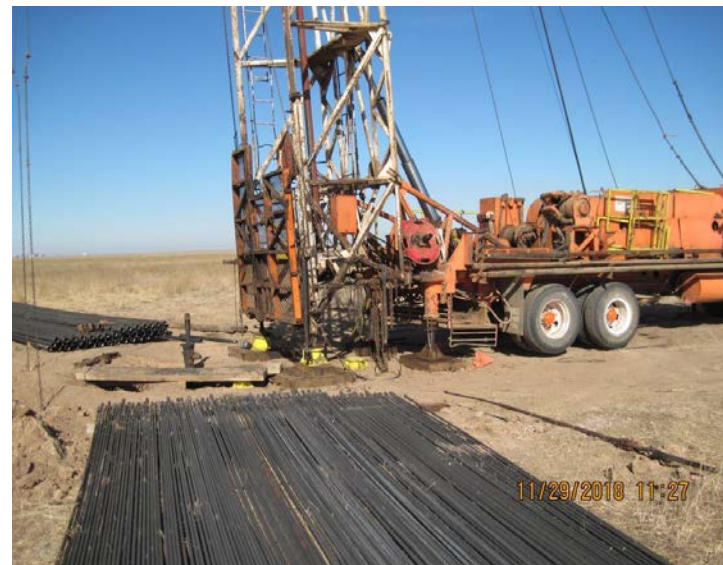
2. Workover rig, Lone Star Rig 1
