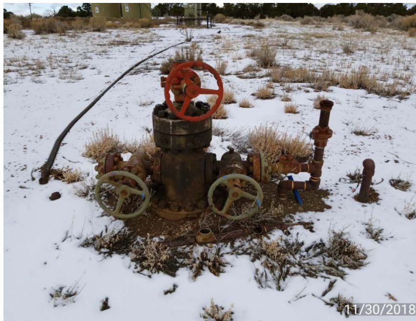
Photo 3. Well disconnected from battery.
