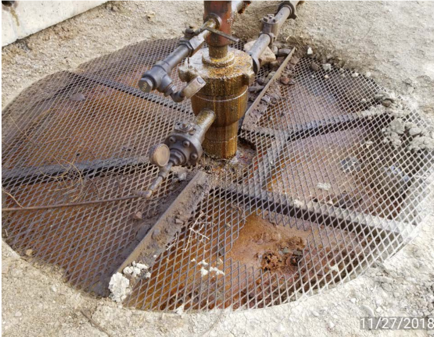
Photo 7. Cellar filled with fluid with 6" of free board.
