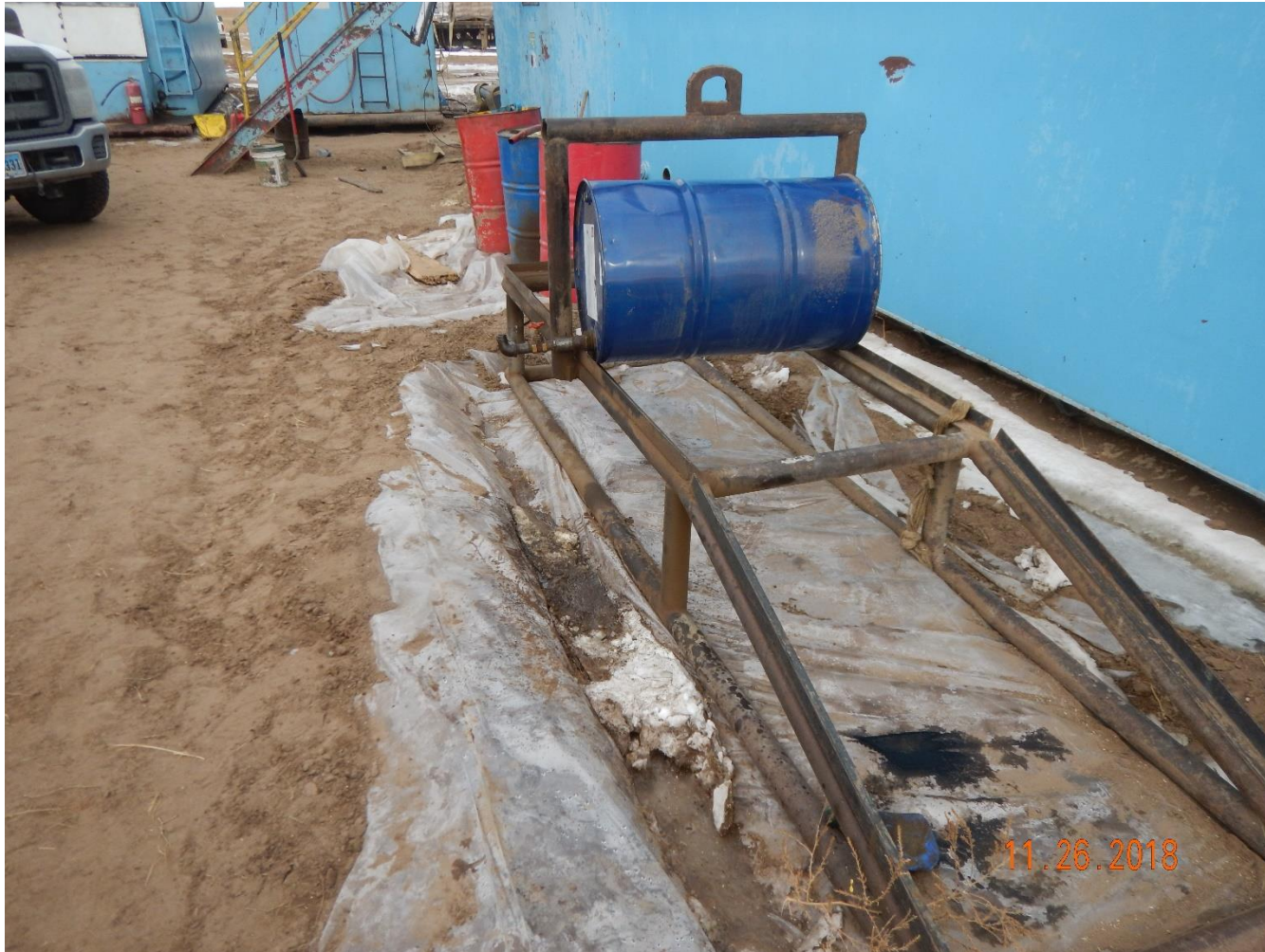
Photo 20: Photo taken from the west end of the drill rig. Photo shows various materials/barrels that do not appear to be within sufficient containment. Plastic material does not appear to be thick/sturdy enough to tolerate abrasions/tears/cuts/etc...
