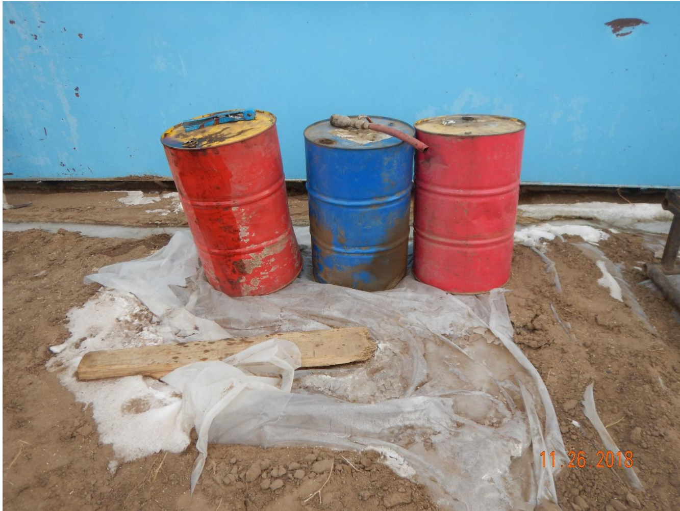
Photo 21: Continued from photo 20. Photos shows barrels with insufficient secondary containment. This is improper materials management.
