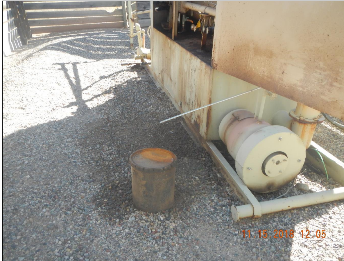
Stained ground surface around separator by pump jack.
