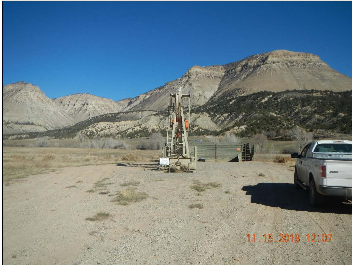
Pump jack with fenced separator behind.
