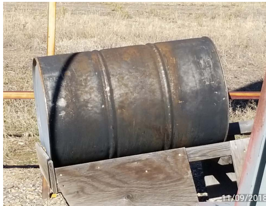
Photo 4. Barrel without label or containment next to wellhead.
