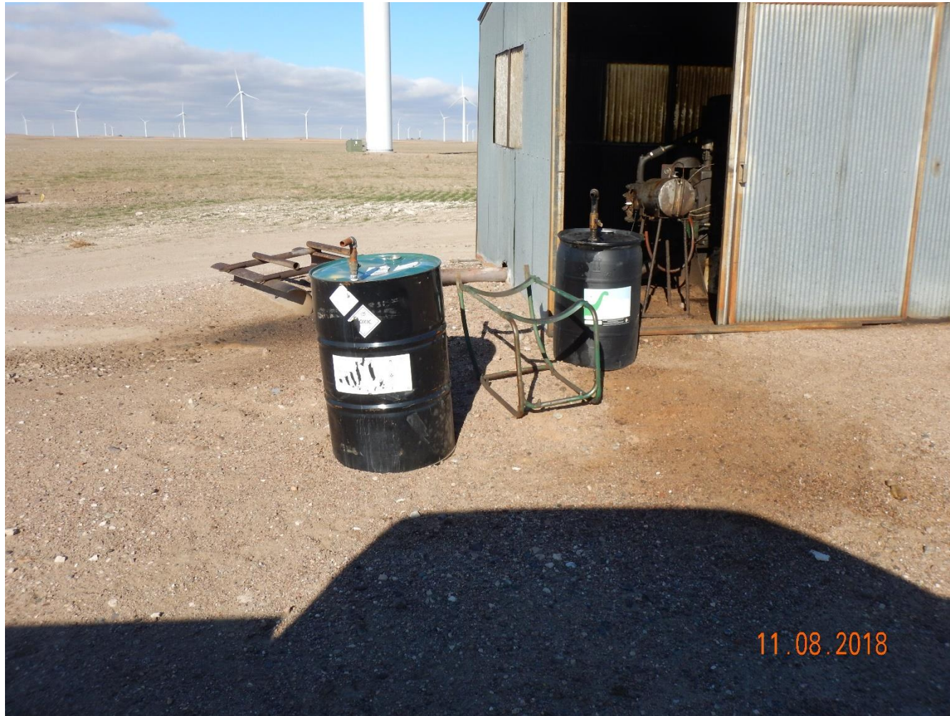
Photo 1: Photo taken from well location, facing north. Previous inspection required barrels to be placed into secondary containment. Photo shows barrels have not been placed into secondary containment.
