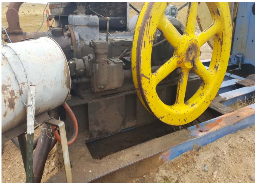
Photo #3 Accumulations of lube oil at base of pumping unit
