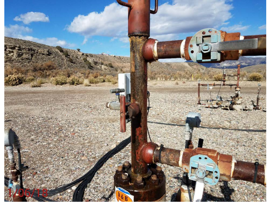
Location Photo #10, Mechanical condition of lubricator on wellhead
