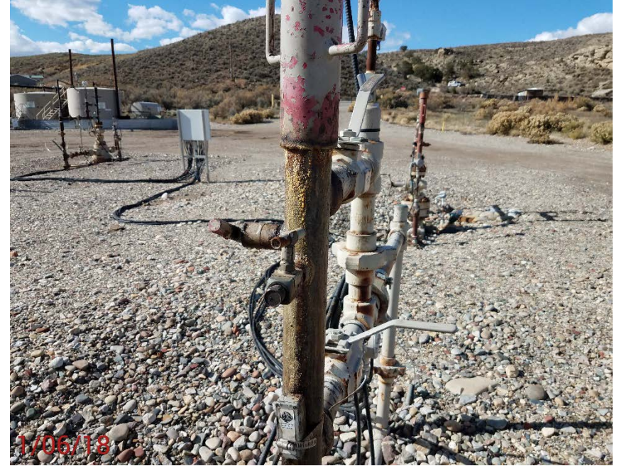
Location Photo #8, Mechanical condition of lubricator on wellhead.
