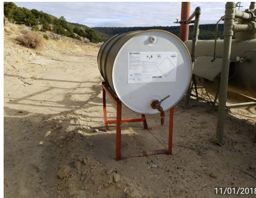
Methanol container without secondary containment
