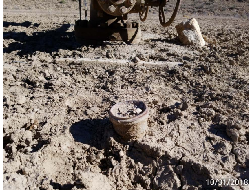
Riser not capped or lock out tagged out
