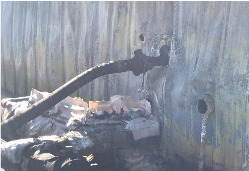
Photo of C7 Skid flex discharge line exiting north wall above the suction line
