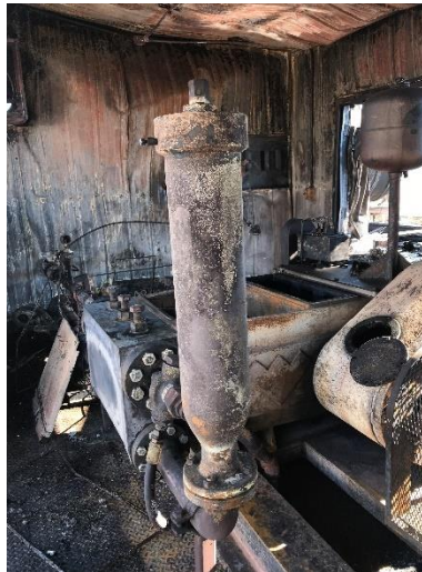
Triplex damage to the flow line pass through chamber of the C7 Triplex Pump.
