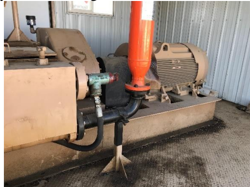
C5 Discharge Line above Suction Line out/in of C5 Pump Triplex Pump Top Inspection Cover and handle is visible in background
