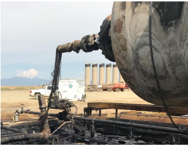
Photo 5: C7 Separator Closeup of Suction Hose Remains
