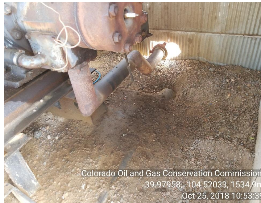
Photo 2 stained soil around PU motor
