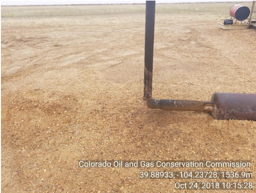
Photo 3 Stained soil PU exhaust pipe
