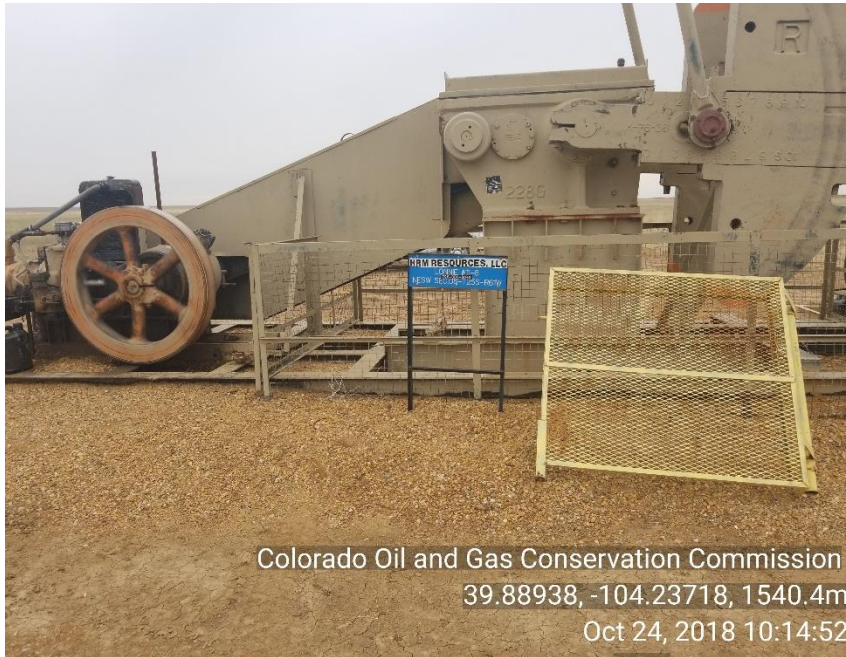
Photo 1 PU unused equipment fly wheel guard
