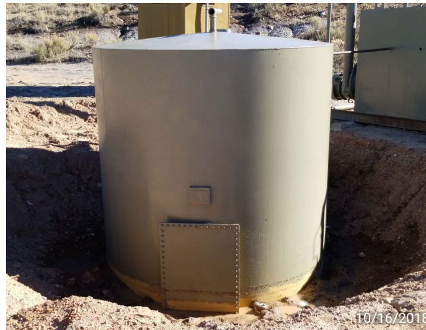
Tank without label for NFPA, capacity, and contents.
