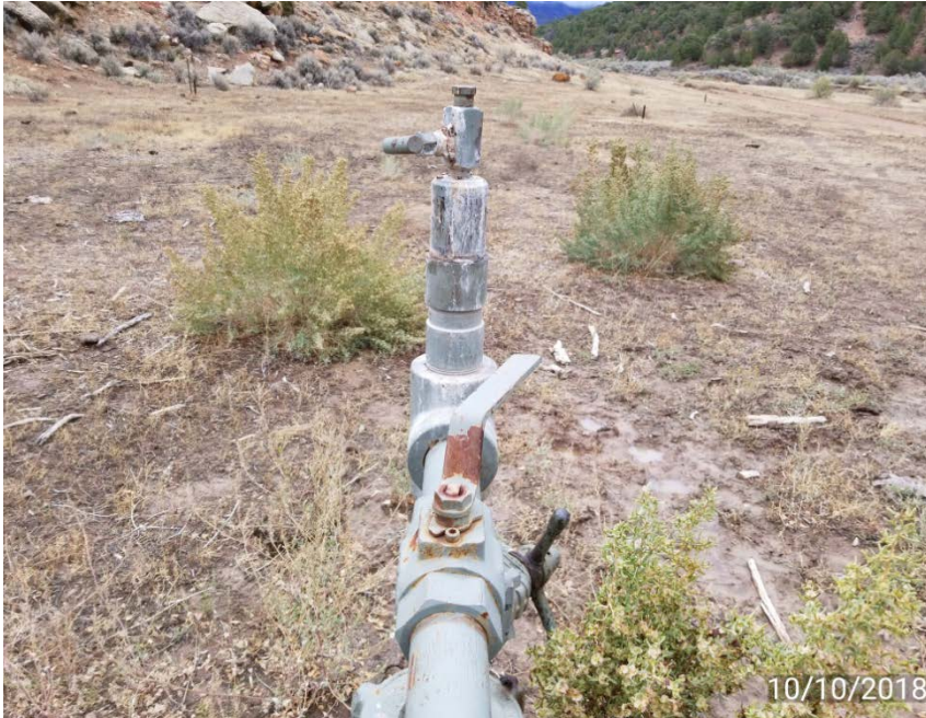
Tubing valve partially open
