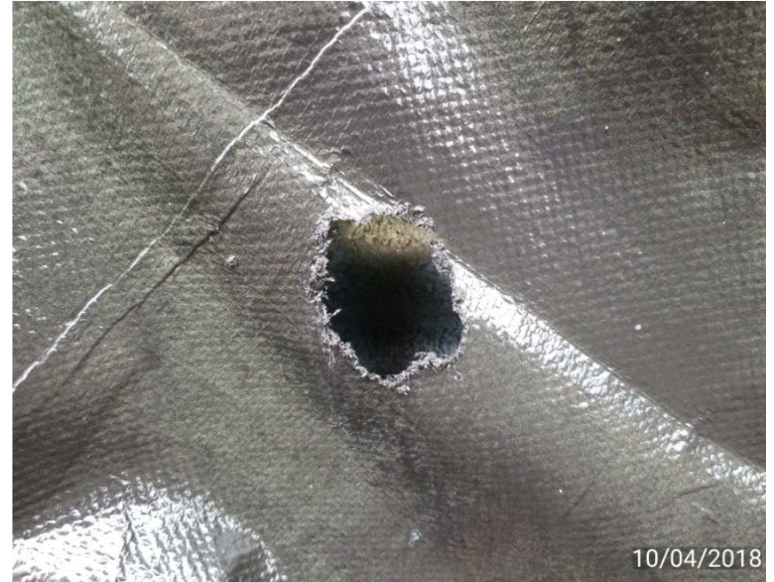
1 of 8 holes in tank battery berm liner
