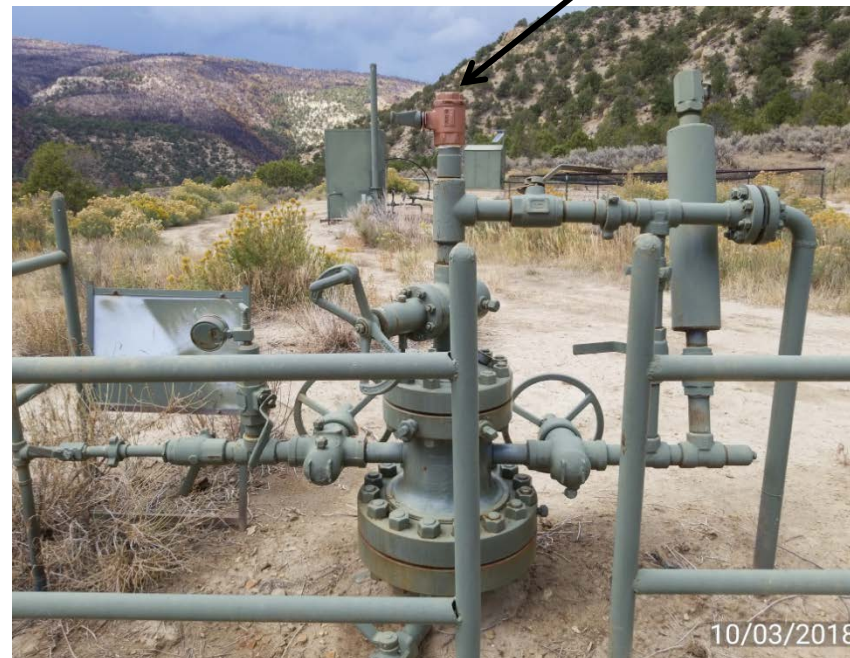
Tubing gas venting through valve
