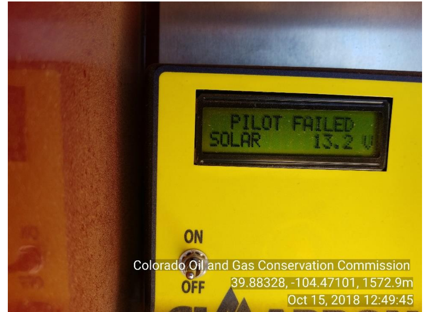
Photo 6 Pilot failure to ECD
