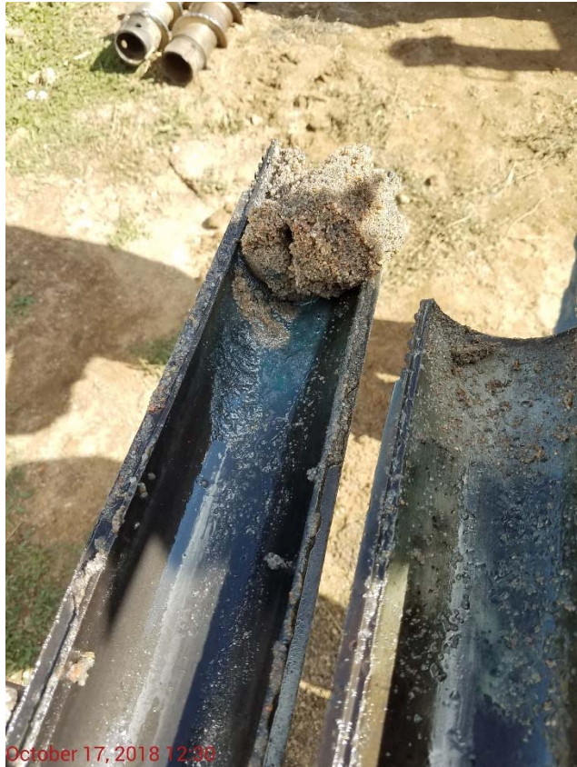
Photo 1 – Photo of continuous sampler at BH03, 9-14' below surface. Note low recovery of material in sampler, saturated sand, and hydrocarbons in sampler barrel.
