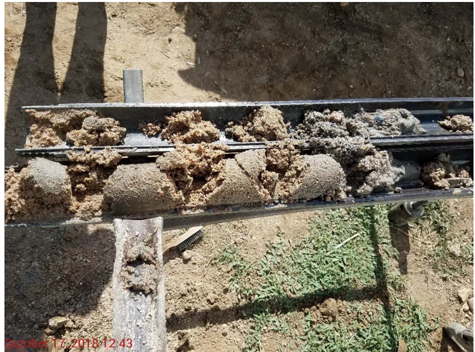
Photo 2 – Photo of continuous sampler at BH03, 19-24' below ground surface. Top of sampler is to right of photo. Approximately 50% recovery of material in this sample. Shallower material exhibits impact. Deeper material to left appears non-impacted.
