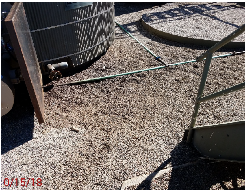
Location Photo #9, Stained rock in battery containment.
