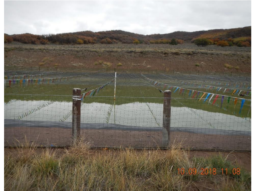
Gauge stick in pit #4 read approximately 9.5'.
