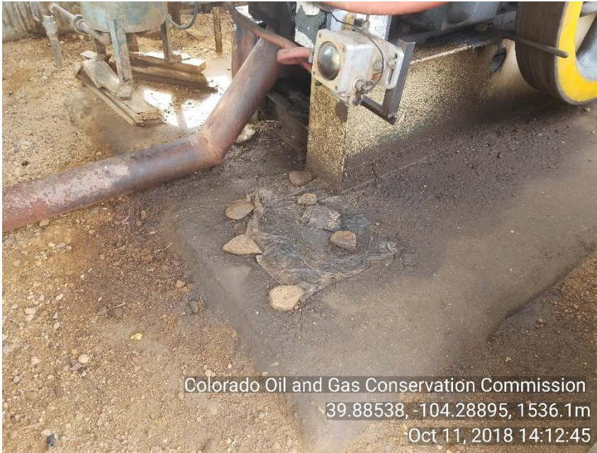
Photo 7 stained soil PU motor
