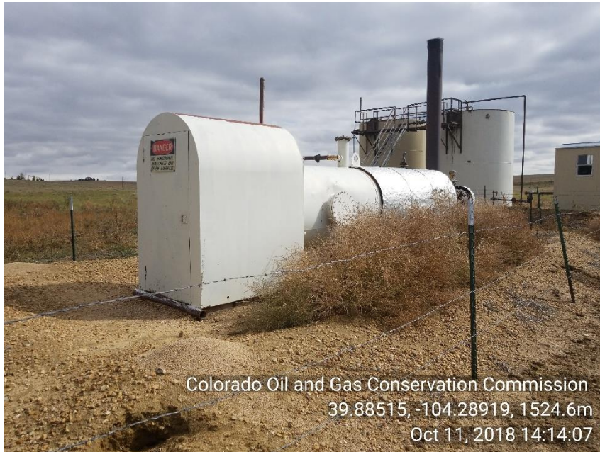
Photo 7 stained soil PU motor
