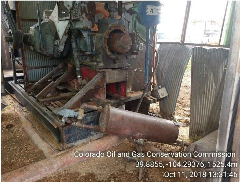
Photo 5 PU house caved in wall and knocked over fuel pot
