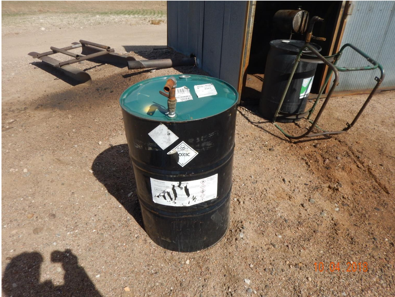
Photo 2: Photo taken at well location. Photo shows two (2) barrels without secondary containment.
