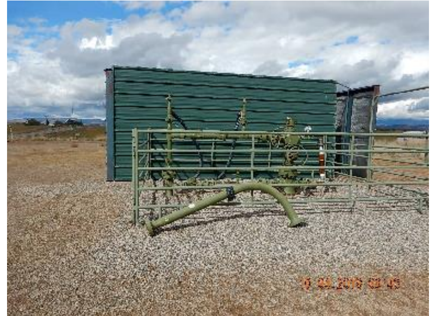
Photo 2: Disconnected pipe at wellhead.
