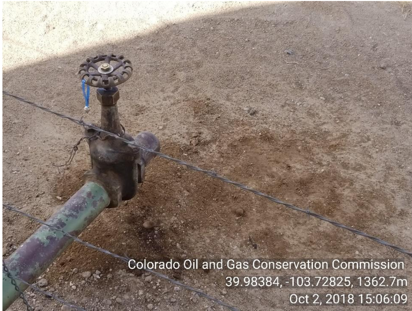
Photo 5 Stained soil under crude oil load out line
