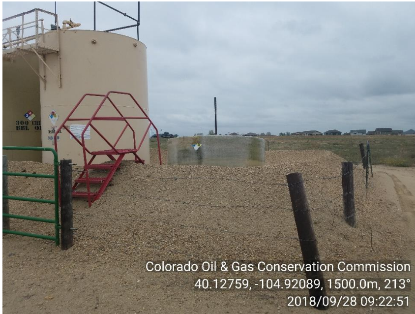
PHOTO 3: TANK WITHOUT SIGN OR MARKING
