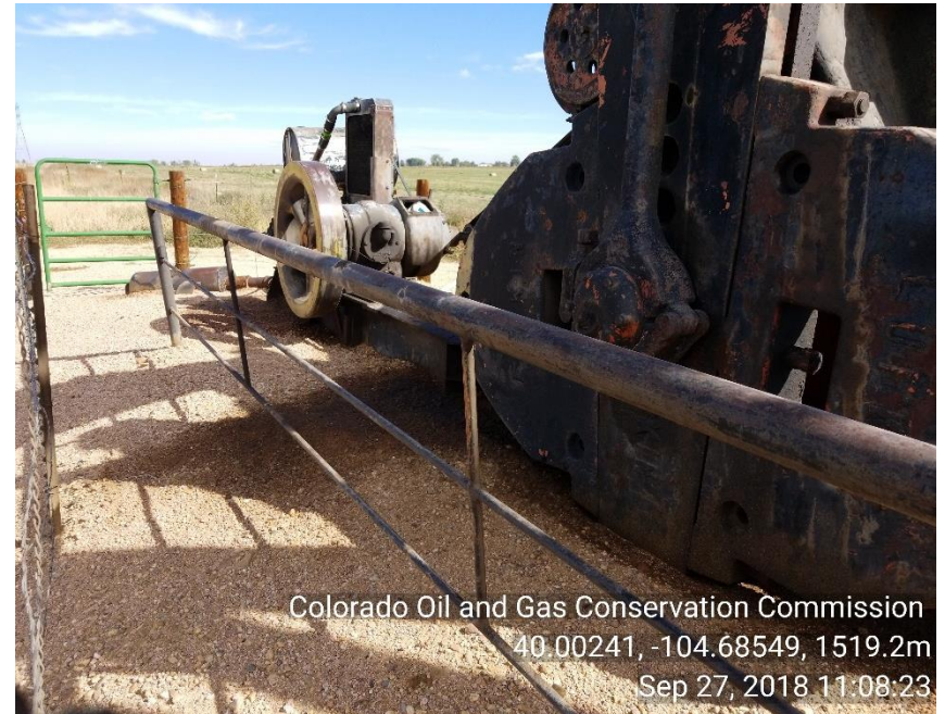
Photo 2 Oil stain around PU
