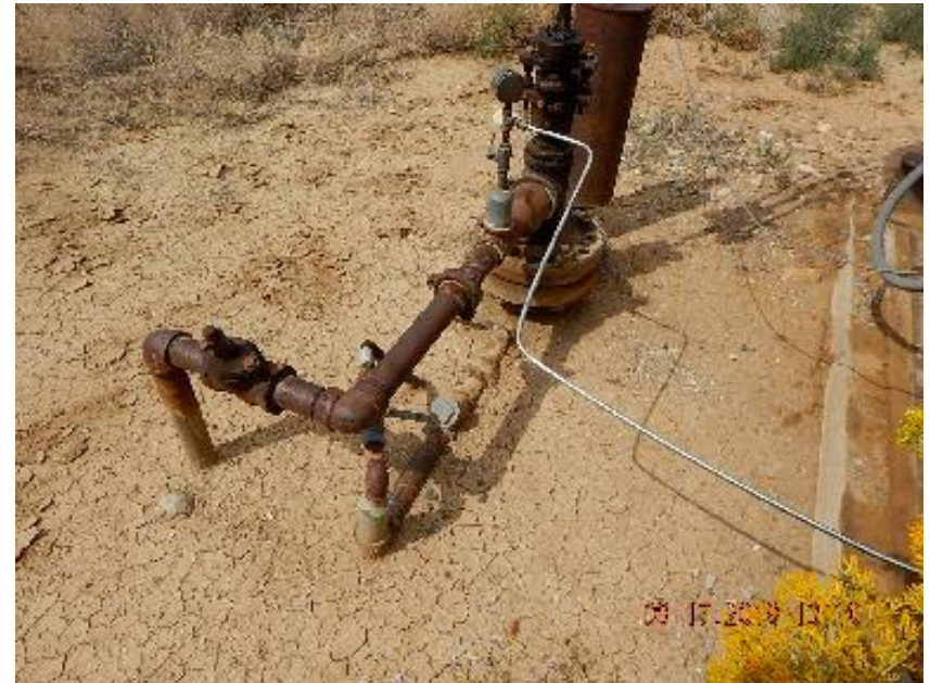
Photo 2: Flow lines at wellhead.
