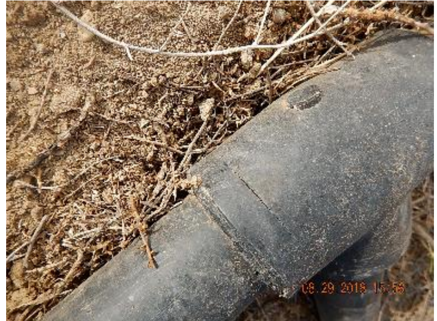
Photo 8: Closer view of split in poly line.
