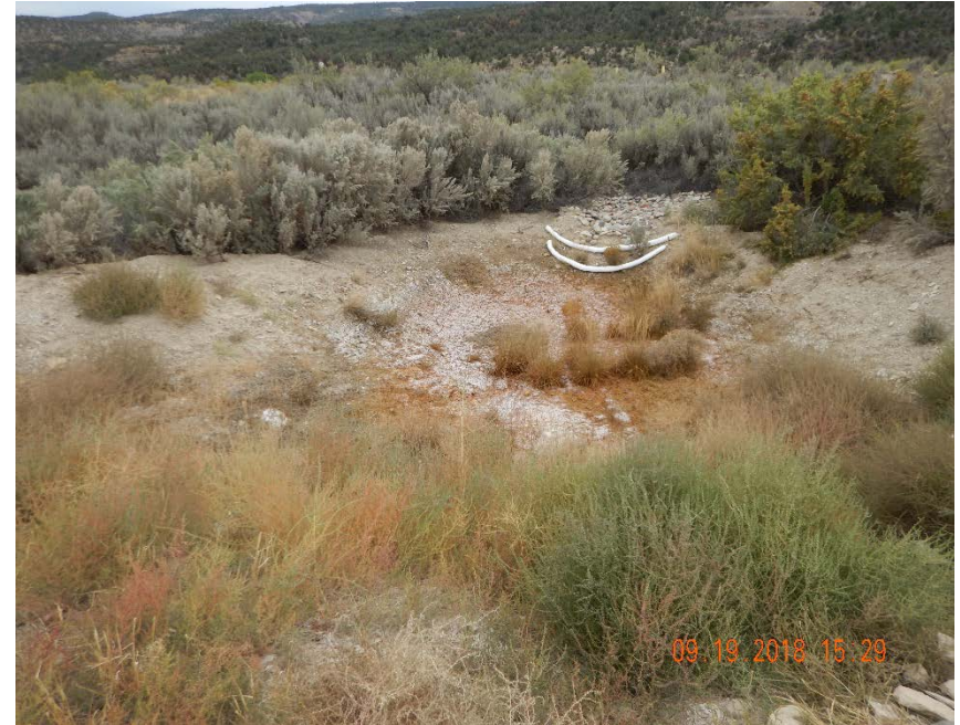
Photo #14 – Sediment trap located at terminus of stormwater ditch was also impacted by produced water released during Spill/Release ID #457570.
