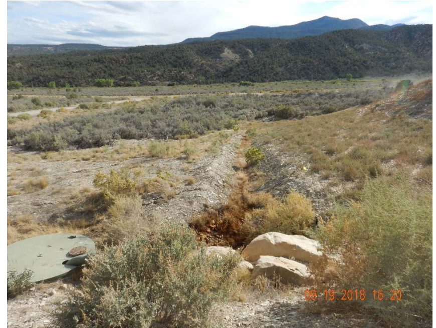
Photo #10 – 10" poly line from previous photo leads into stormwater ditch on south side of lease road through a culvert. Produced water impacts from Spill/Release ID #457570 extend into this ditch for approximately 200'.
