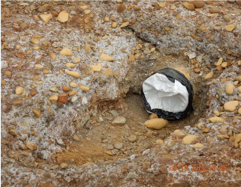
Photo #3 – View of exposed, severed 10” poly line that was source of Spill/Release ID #457569.
