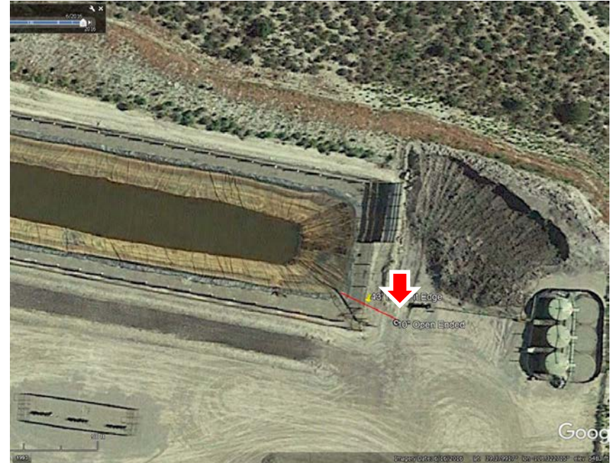
Photo #2 – Google Earth 2016 aerial photo provided by operator depicts location of severed 10" poly line in relation to historical Pit ID #432420. COGCC records indicate that pit was abandoned by previous operator in November 2017. See Remediation Project #10495 for additional information.
