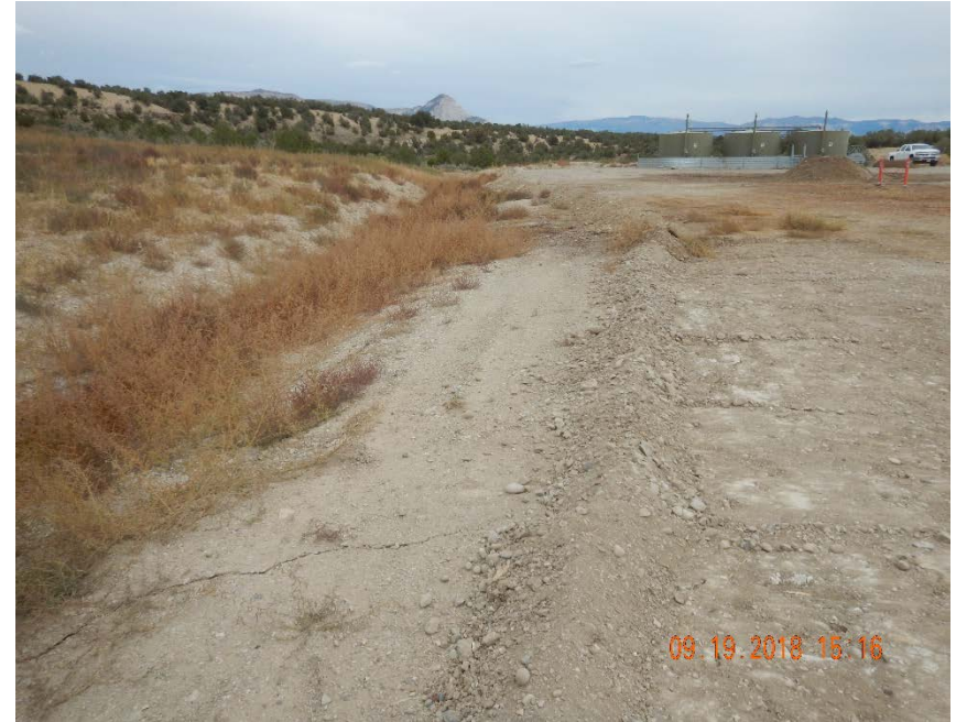
Photo #4 – Produced water released from 10” polyline flowed NW into stormwater ditch overlying former pit location. Operator constructed containment berm along ditch.
