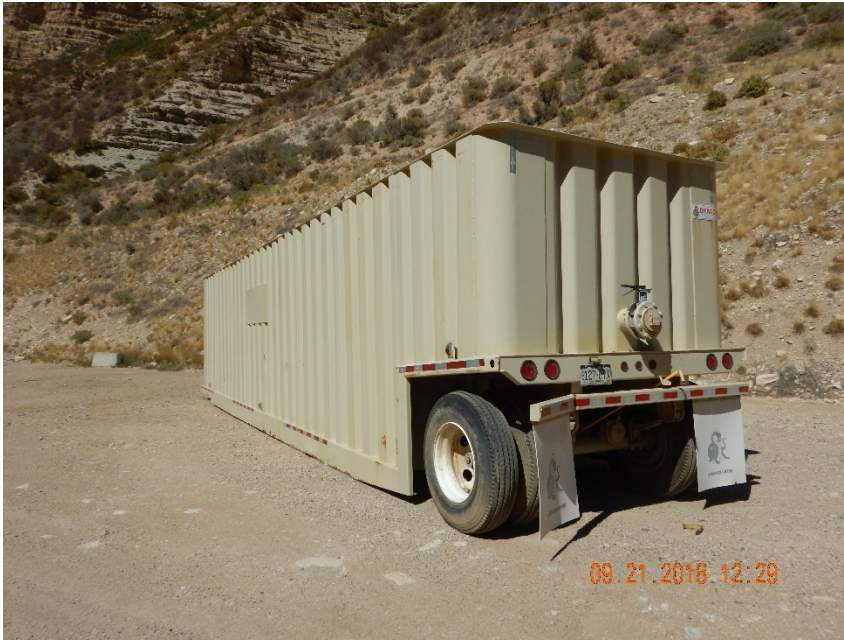
Photo #5 – Frac tank located at NE corner of pad.
