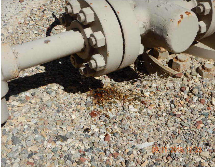
Photo #9 - Localized accumulation of oil-stained soil at K22 04A-27 WF04A-27 K22 596 wellhead.
