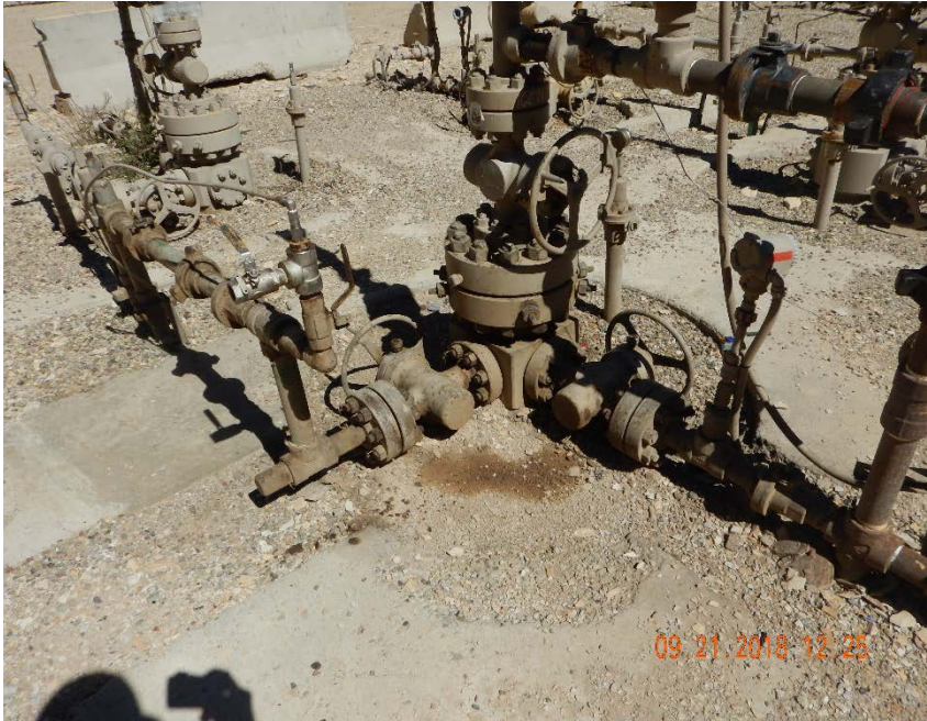
Photo #11 - Localized accumulation of oil-stained soil at wellhead. Note that this wellhead did not have a sign attached.
