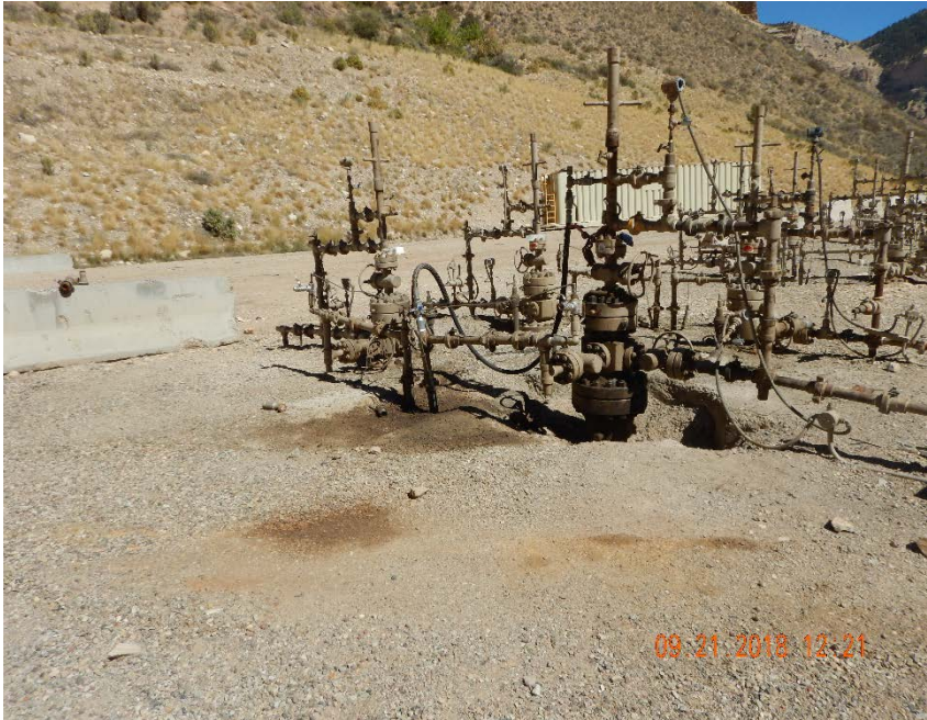
Photo #7 – Localized accumulation of oil-stained soil at WF 04B-27 K22 596 wellhead.
